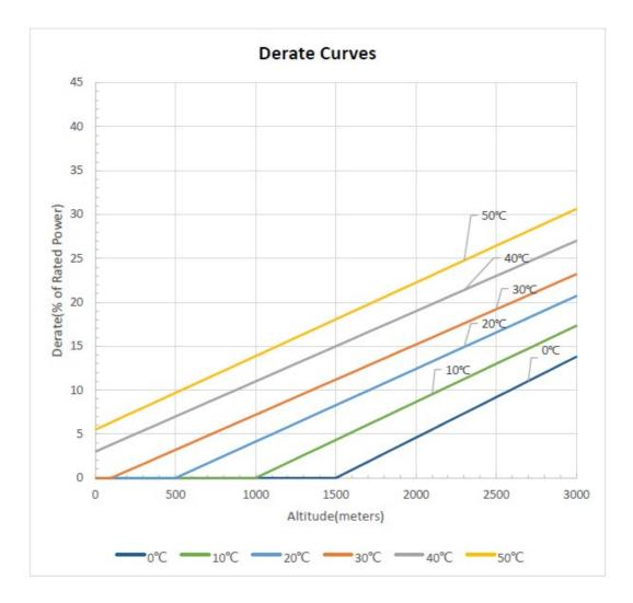
\* Estimating the effect of altitude & temperature for the engine output relative to ISO reference condition at sea level.
